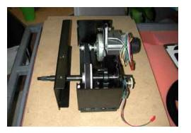
Slide the front plate off the assembly and off the shaft. Then remove the belt from the two pullys of the motor and the shaft.
